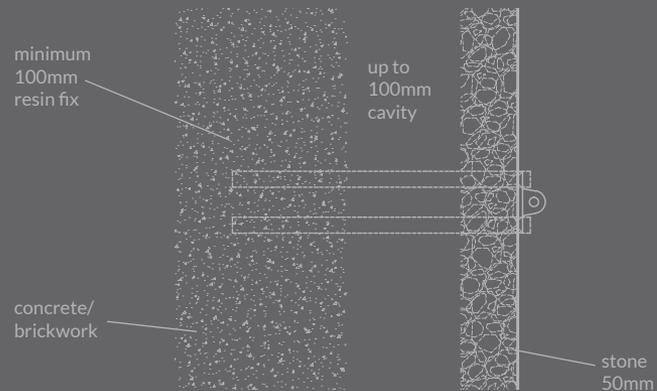
**Fixing:** Resin bolt / studding M6
