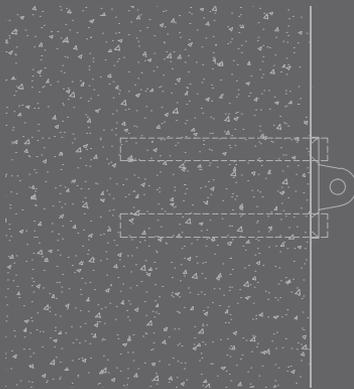
**Fixing:** Anchor bolt
