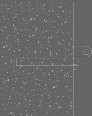
**Fixing:** Anchor bolt
