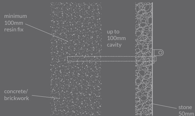
**Fixing:** Resin bolt / studding M8
